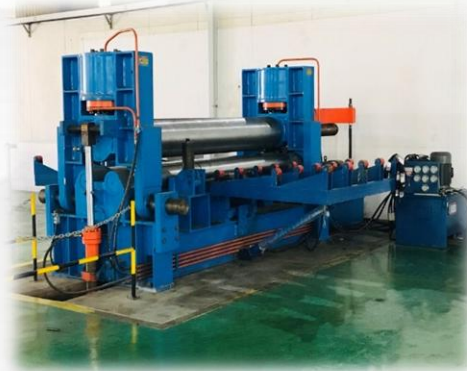
HYDRAULIC ROLLING MACHINE 25X2500
